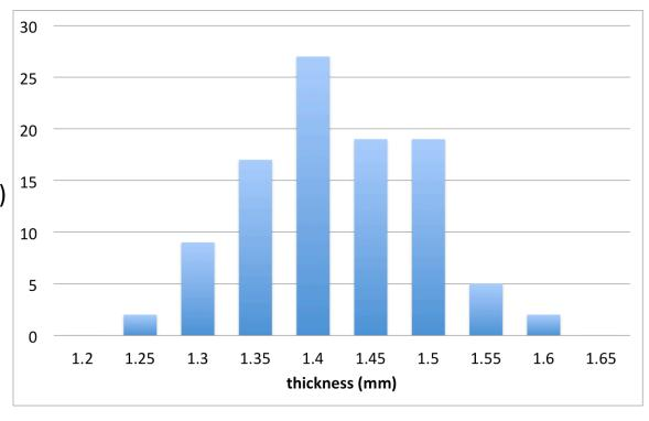
The thickness of a new penny is designed to be 1.52mm, considerably thicker than the average of the sample above. The shift in the distributions suggests some kind of systematic error in the measurement. In this case, the two faces of the micrometer are not exactly parallel; on one side the micrometer, where we made all the measurements, it measures a little too low.
